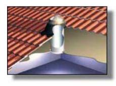
Aluminium gives a slightly 'bluer' quality to the light. Diffusers should be fitted to tubular skylights to reduce glare and throw the light over a broad area.
